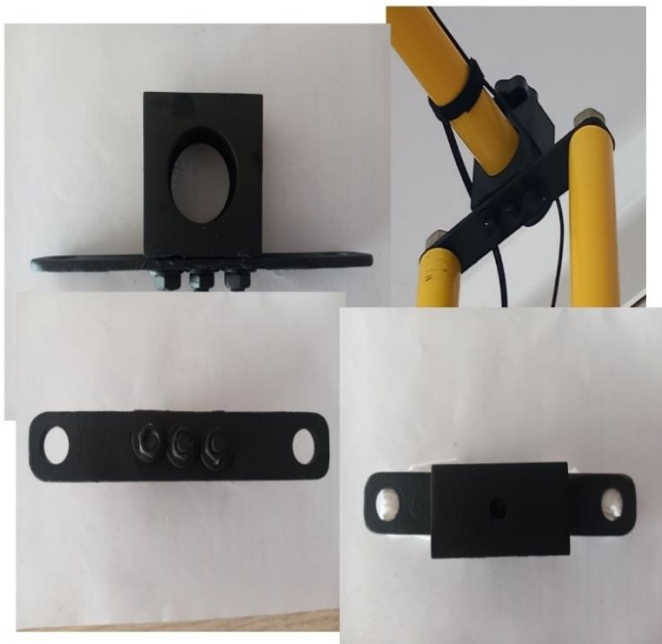
Fig. 4 : connection joint between the horizontal arm and the main structure.
