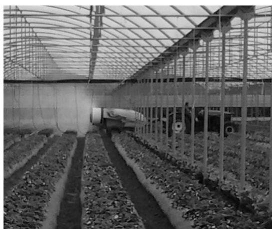
Figure 4. hand sprayer and air-blast application method The tractor stood outside the greenhouse entrance while the spray operator held the spray lance at the end of a high-pressure hose connected to the tractor pump. The spray operator walked in plant rows spraying. He moved the lance continuously up and down, with the spray nozzle facing upwards, to the top of the plants, and with the nozzle spraying downwards, and back again.
