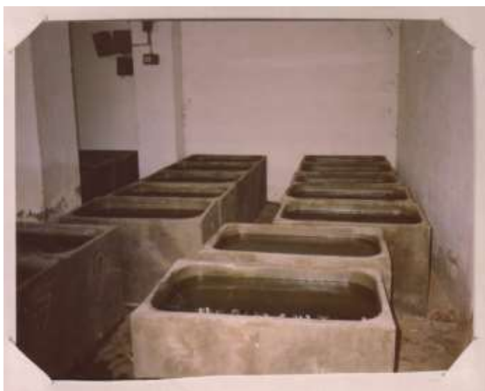
Figure 1.2: Showing the experimental unit consisting cement cisterns of 185 lit. capacity
