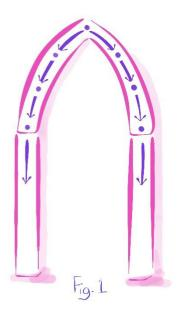
Is more efficient in this application than a semicircular arch (figure 2)
