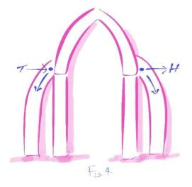
Because a Gothic arch transfers weight with a smaller horizontal component and a larger vertical component (Huber, 2009). In quantitative terms L in figure 3
