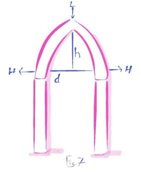
Demonstrates the problematic issue where d is the half the span of the arch and h is the height and H represents the horizontal component of the thrust that is generated at the point of convergence (Huber, 2009) – across the perineal area outward to the femoral neck:
