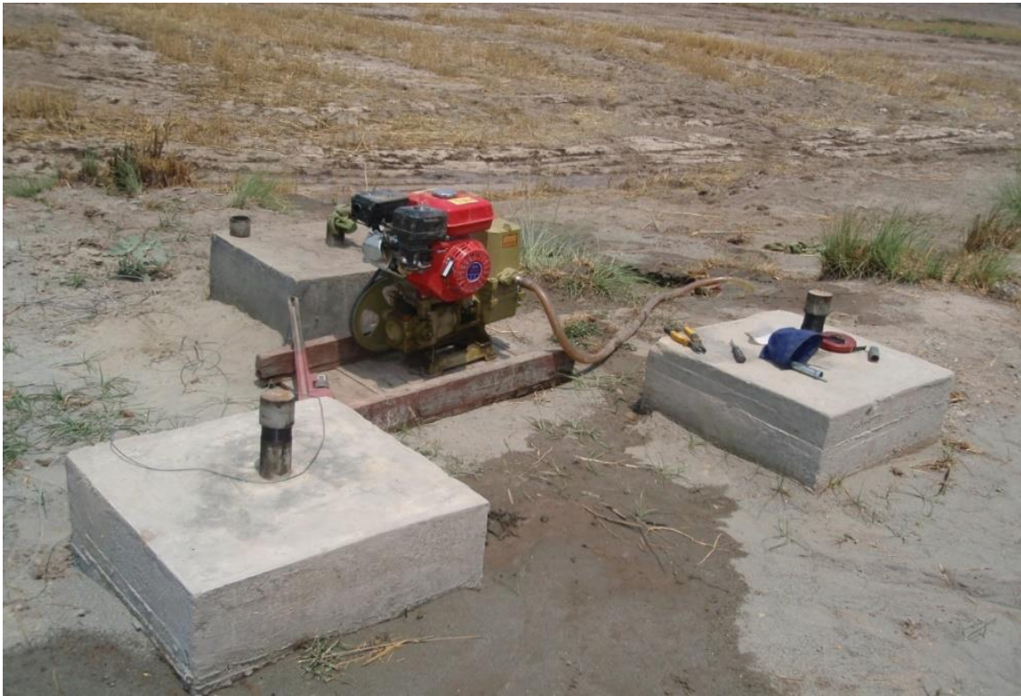
Figure 6: Battery of three piezometers along Ravi River at 50, 100 and 150 ft depths at Mohlanwal
